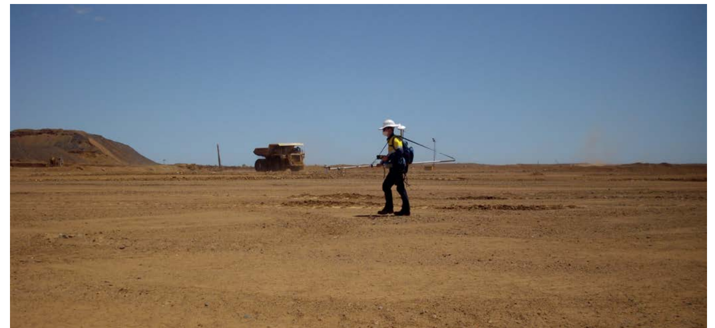
Ore body delineation using high resolution magnetometer profiling
